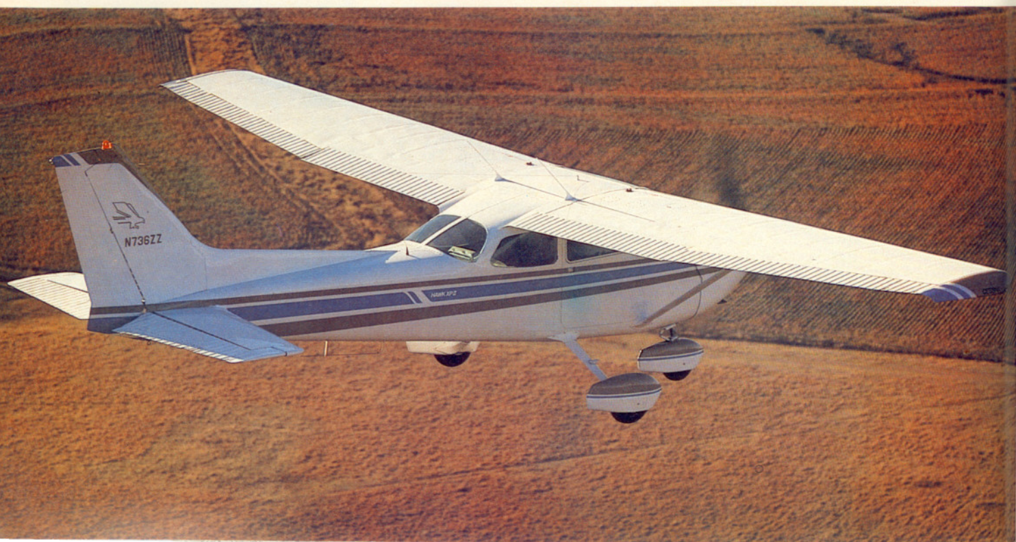
With a 66-gallon useful fuel capacity in optional integral fuel cells, the Hawk XP offers a maximum 938-statute-mile range with 45-minute reserve.
