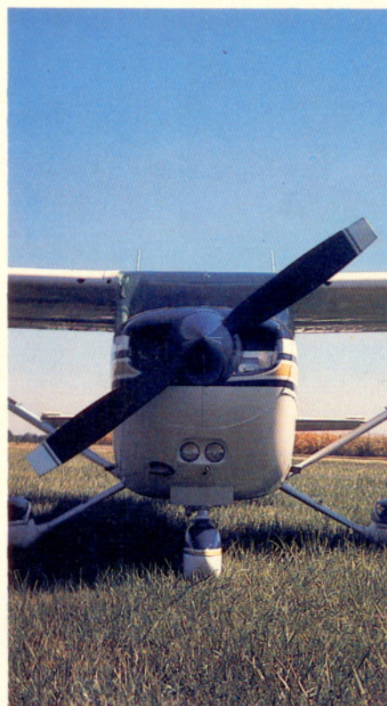
It may look like a Skyhawk, but the Hawk XP's beefier engine cowl covers a 195-hp Continental engine that teams with a constant-speed prop for extra performance.
